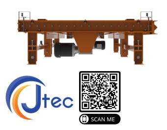
The Powered Roller CarryMatic Station, normally a CDLR type conveyor station, performs automated material transfers with CarryMatic carts and with other Powered Conveyor Sections, within a CarryMatic System. Stations are equipped HMI control panels with E-Stop, load present sensors, and cart alignment sensors. Guards and additional E-Stop positions are also available. These stations can be used for both loads and unload transfer to and from the CarryMatic carts.
