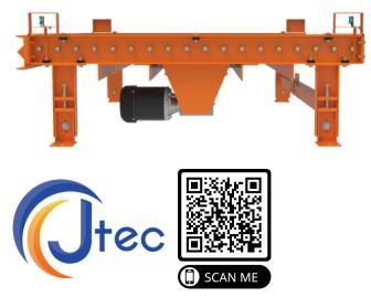
The Powered Roller CarryMatic Station, normally a CDLR type conveyor station, performs automated material transfers with CarryMatic carts and with other Powered Conveyor Sections, within a CarryMatic System. Stations are equipped HMI control panels with E-Stop, load present sensors, and cart alignment sensors. Guards and additional E-Stop positions are also available. These stations can be used for both loads and unload transfer to and from the CarryMatic carts.
